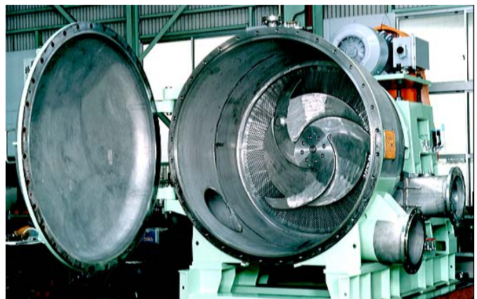
Contaminants Handling of AHP; Dumping Screen PEA1400-B and Screw Separator
