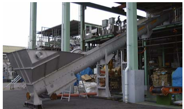
Contaminants Handling of AHP; Dumping Screen PEA1400-B and Screw Separator
